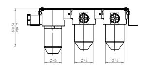
The producer set and guarantee the termostatic valve at 38°C (see position on the drawing). Maximum temperature at 3bar 49°C.
